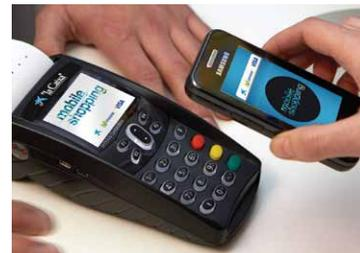
The project uses Near Field Communication short-wave wireless communication technology between the phone and the reader terminal. A Samsung Star Touch phone was deployed with a secure mobile SIM chip inside, which effectively acts as a Visa card.
